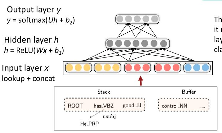
The hidden layer re-represents the input — it moves inputs around in an intermediate layer vector space—so it can be easily classified with a (linear) softmax
