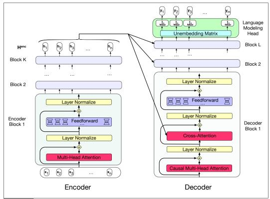
Figure 13.6 The transformer block for the encoder and the decoder. The final output of the encoder  $\mathbf{H}^{enc} = \mathbf{h}_1, ..., \mathbf{h}_n$  is the context used in the decoder. The decoder is a standard transformer except with one extra layer, the **cross-attention** layer, which takes that encoder output  $\mathbf{H}^{enc}$  and uses it to form its  $\mathbf{K}$  and  $\mathbf{V}$  inputs.
