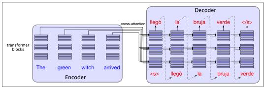
The encoder-decoder transformer architecture for machine translation. The encoder uses the transformer blocks we saw in Chapter 8, while the decoder uses a more powerful block with an extra crossattention layer that can attend to all the encoder words. We'll see this in more detail in the next section.
